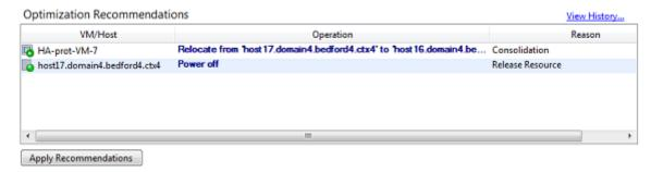
This illustration shows a screen capture of the Optimization Recommendations list, which appears on the **WLB** tab. The **Reason** column displays the purpose of the recommendation. The **Operation** column displays the behavior change suggested for that optimization recommendation. This screen capture shows an optimization recommendation for a virtual machine, HA-prot-VM-7, and a host, host17.domain4.bedford4.ctx4.
